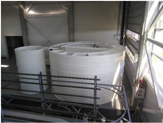
Biological reactor and the excess sludge tank ready for dispatch from the factory
