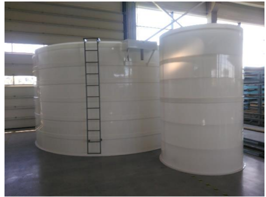
Biological reactor and the excess sludge tank ready for dispatch from the factory
